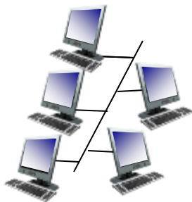
shared wire (e.g., cabled Ethernet)
